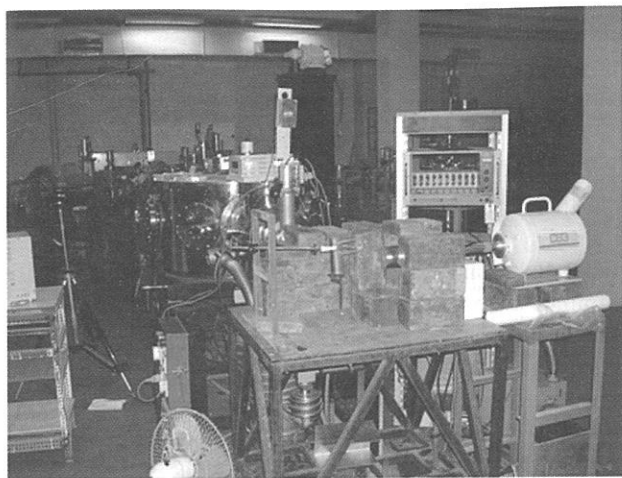
Fig. 4 Photograph of Photon Induced Positron Annihilation (PIPA) facility at FOTIA for volumetric assay of defects in large engineering materials
