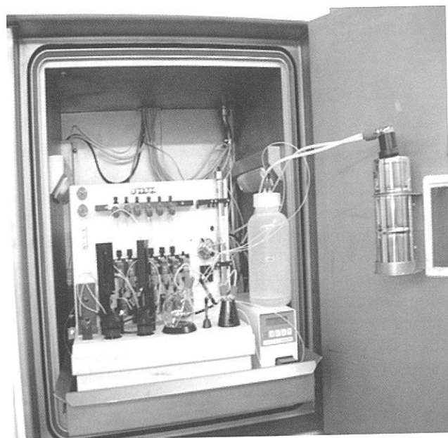
Fig. 3 A general purpose ^{18}\text{F} -radiofluorination module for nucleophilic reactions. It is provided with a semi-prep HPLC. The liquid nitrogen trap in a Dewar's flask can be seen on the right. This module can be used for making a variety of ^{18}\text{F} -labeled compounds. It has a semi-prep HPLC for purification of the final product, but can be by-passed if solid-phase extraction cartridges are used.
