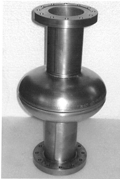
Fig. 6 First solid Nb single cell cavity (left) fabricated by a team from IUAC & RRCAT and first results (right) obtained with the Vertical Test Stand at Fermilab.
