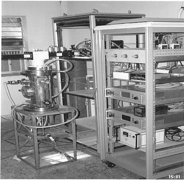
Microwave Plasma CVD Reactor (2.45 GHz, 2 kW) for Oriented Diamond Thin Film Deposition
