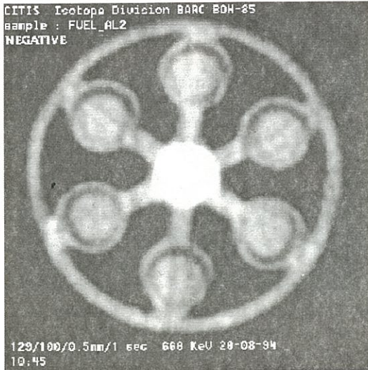
Fig. 3 A cross-section of an experimental fuel pin assembly (end cap)
