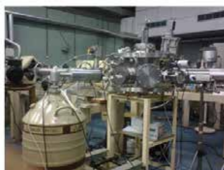
Figure 3. Proton Induced X-ray Emission (PIXE)/ Particle-induced Gamma-ray Emission (PIGE) Line with experimental chamber, Facility for: PIXE/PIGE, Scattering & Nuclear Reaction Analysis (NRA).
