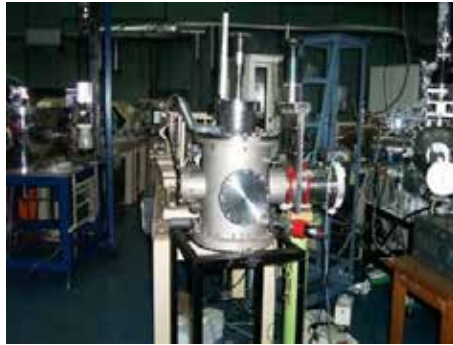
Figure 4. Implantation beam Line, Facility for Ion Implantation & Ion Irradiation
