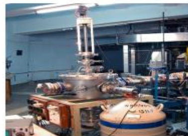
PIXE Facility : Scattering Chamber & Si(Li) detector
