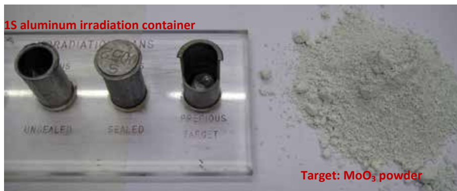
Figure-1. Encapsulation of MoO 3 target in standard 1S aluminum irradiation container
