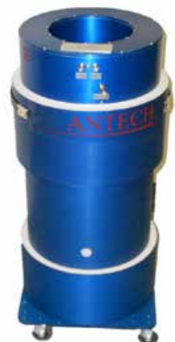
HLNCC High Level Neutron Coincidence Counter
