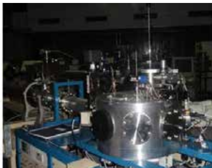
Figure 2. Rutherford Back Scattering Beam Line with experimental chamber, set up for RBS, Ion Channeling & Elastic Recoil Detection Analysis (ERDA).
