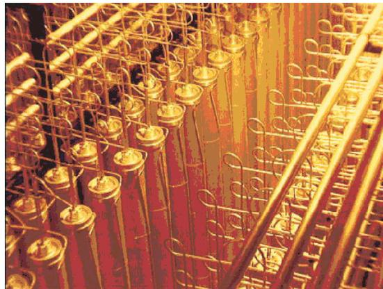
Fig. 6 A view of part of a URENCO Gas Centrifuge cascade (from site <http://www.uic.au/graphics/centrfge.jpg>)
