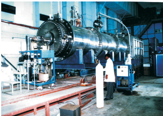
Fig. 6 A View of KALI 5000 for Flash X rays Radiography.
