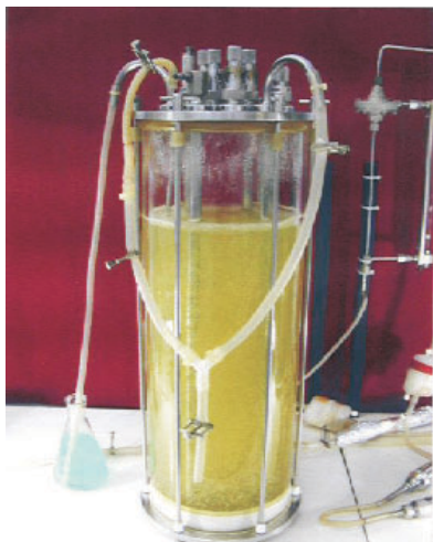
Fig. 1 Scale-up of Catharanthus roseus cell cultures in 20 L airlift bioreactor
