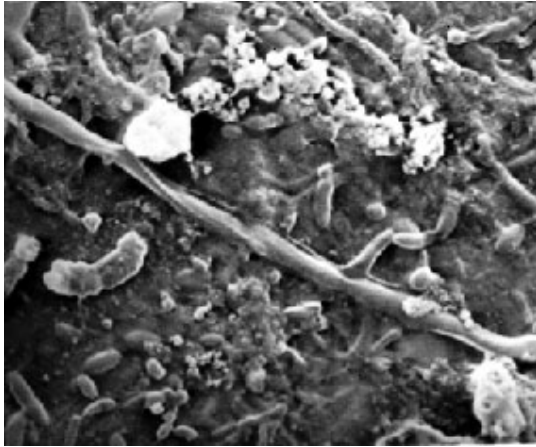
Fig. 1 SEM pictures (X 1725) showing a mix consortium of micro -organisms, diatoms and filamentous forms in a freshwater biofilm
