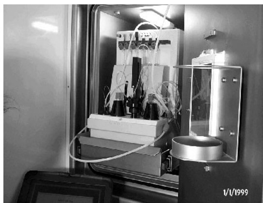
Synthesis module for [ 18 F] FDG
