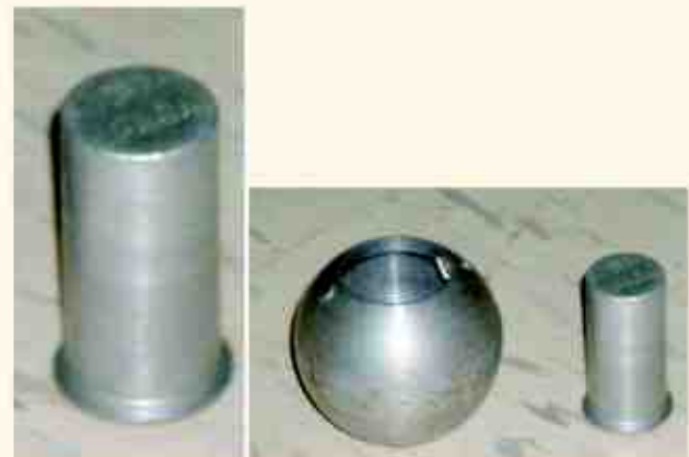
Figure-2: Tray rod capsule & Self Serve Aluminium Sphere and capsule
