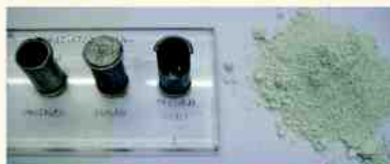
Fig. 1. Standard 1S Aluminum cans, target encapsulation and a typical target
