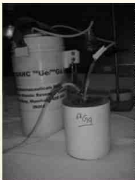
Figure 5: 'BARC' ^{68}\text{Ge}/^{68}\text{Ga} generator supplied to TMH, Mumbai for clinical studies.
