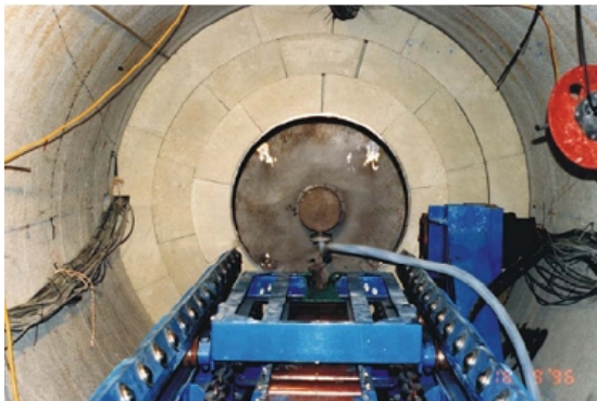
Fig. 2 Use of highly compacted clay bricks around waste overpack
